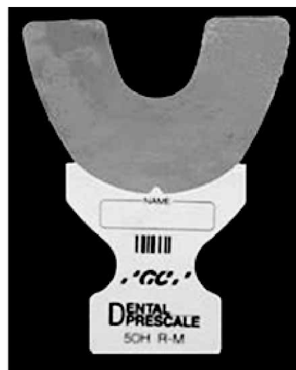
Fig. 1. Fuji film Prescale cut in the shape of a dental arch and film holder
